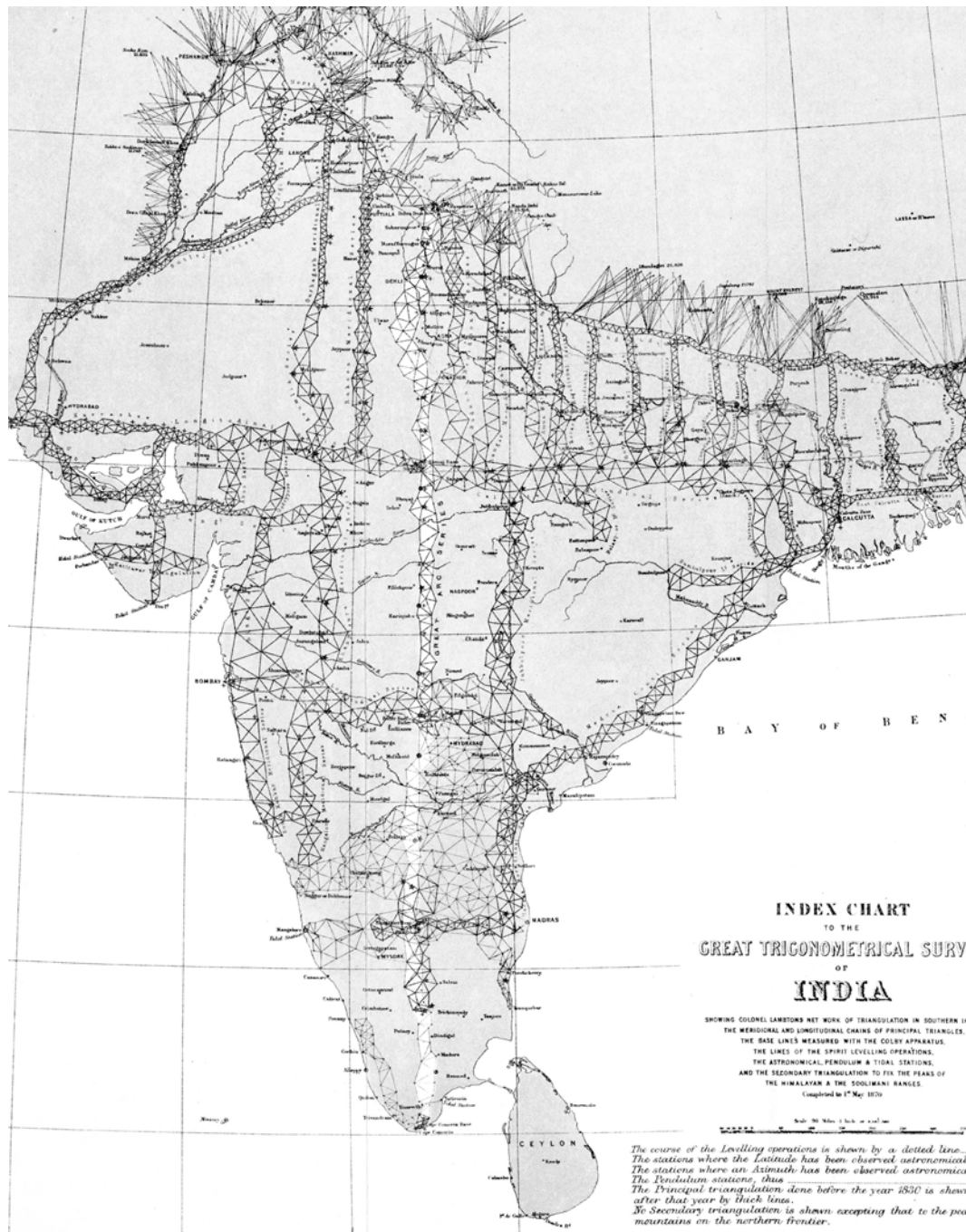
Figure 3-19: A map of the triangulation survey network established across India in the 1800s. Each leg of the triangles, shown here as a single line, is in turn a triangulation survey. This nested triangulation provides reinforcing measurements, thereby increasing the accuracy of the surveyed positions (courtesy NMSI).
