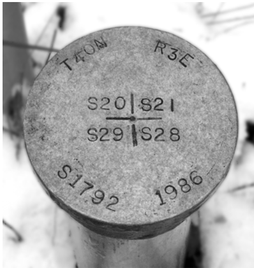
Figure 3-50: A PLSS corner that has been surveyed and marked with a monument. This monument shows the physical location of a section corner. These points are often as control point for further spatial data development.
